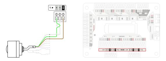
Power to the reader can be supplied using POE or a 12-28VDC external power source. DR40 has a maximum current rating of 1.05 A at 12 VDC, so should not be powered directly by the DC20. Always check the power requirements of the door controller prior to installation. If PoE is not used, an Ethernet connection is required. Refer to Recommended Wire Type and Size table above for more wiring detail.
