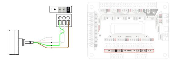
Power to the reader can be supplied directly by the 12VDC power supply in the "WIEGAND" section of the DC20 Door Controller. Alternatively, an external power supply can be used. Note that DR20 requires 8-28VDC with a maximum power of 4.8W. Refer to Recommended Wire Type and Size table above for more wiring detail.
